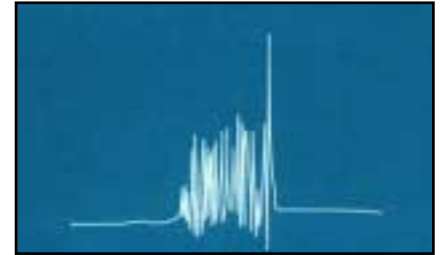
Electrical Noise from Motors
