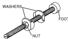
An optional adjustable spindle assembly is ideal for clamping work pieces that vary in height or may be damaged by the steel holddown bar.
