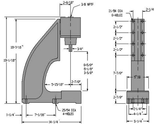
This press combines the AP-400M press stand with a Mead H-122 single-acting cylinder (4" bore, 2 5/8" stroke). Cylinder details are on page 29.
