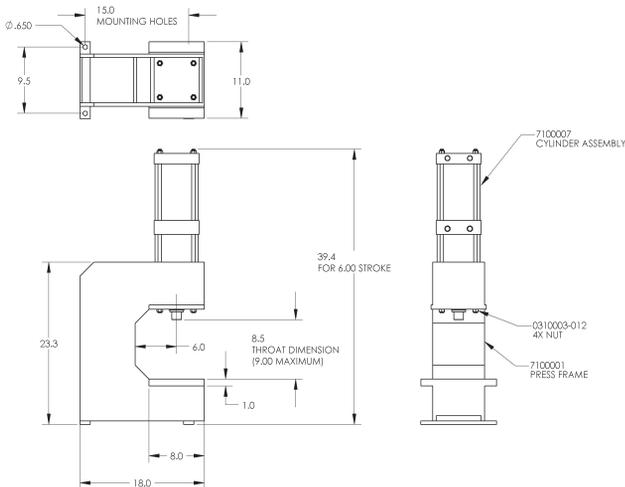
Note: For each inch of stroke overall height increases by 2"
