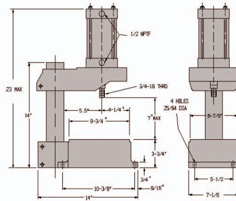
For non-standard double-acting service with strokes up to 4", use pages 14-15 to create a 4" bore cylinder for use with this stand. The PL-400 cylinder-to-stand adapter plate will be required.
