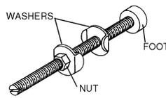
An optional adjustable spindle assembly is ideal for clamping work pieces that vary in height or may be damaged by the steel holddown bar.
