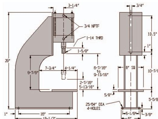
This press combines the AP-600M stand with Mead's #6040303 (H-283, p. 29) single-acting cylinder (6" bore, 3" stroke). A PL-600 cylinder-to-stand adapter plate is required to mount this cylinder.
